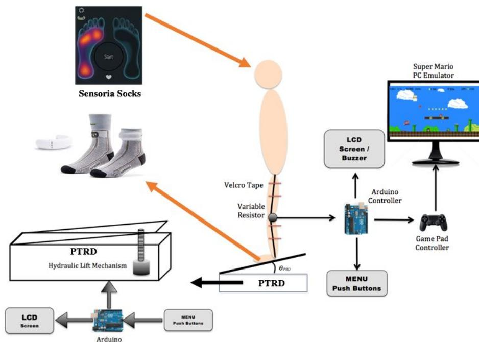
Figure 1 PTRD with Sensoria feedback mechanism
